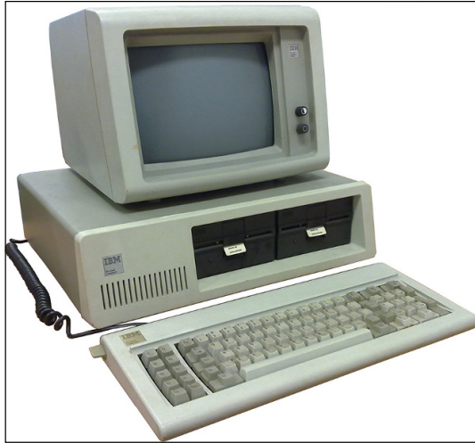
FIGURE 8-3: The first IBM PC, model 5150 with model number 5151 monitor and IBM PC keyboard Photo courtesy of Ruben de Rijcke via Wikimedia Commons
