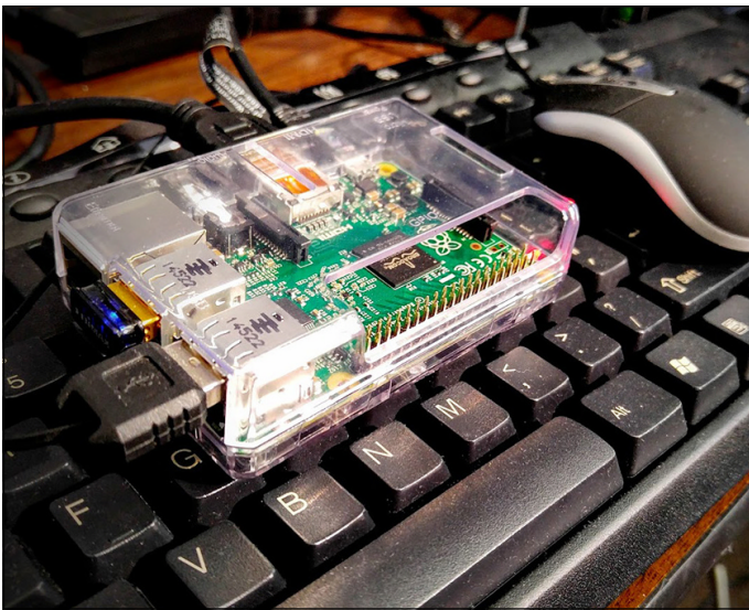
FIGURE 1-3: Peripherals attached to a Raspberry Pi 2 Model B
